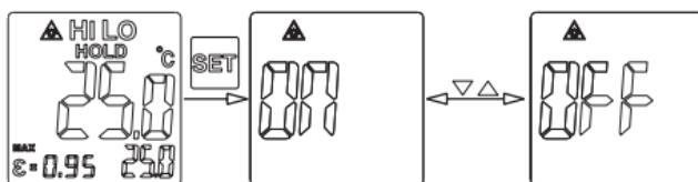
**10. Trigger free measurement setup**
